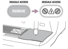
Use a flat-head screwdriver to rotate the right screw counter-clockwise until the valve is fully open. As the valve opens, steam may be released.
